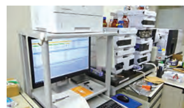
Analysis of micropollutants with a liquid chromatography mass spectrometer
